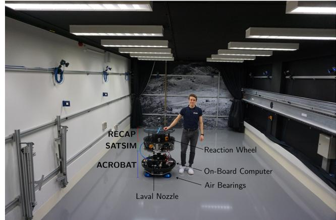
Fig. 1. The first author at the ORGL at ESTEC. An epoxy flat-floor for floating air-bearing platforms, where slight unevenness induces disturbances.
