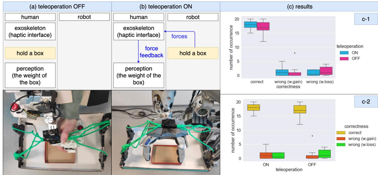
Figure 1 Experimental setup (a,b) and results (c)
