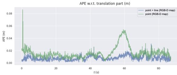
Fig. 5: **The evaluation of re-localization module.** We illustrate the absolute pose error (APE) [m] of all the re-localized images from sequence *freiburg3\_long\_office\_household*, where the x-axis indicates the relative timestamps.
