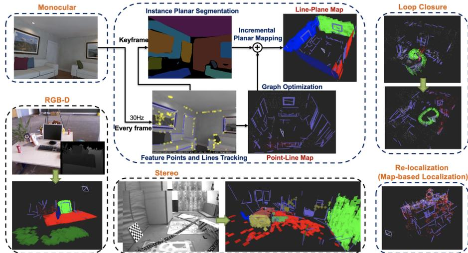
Fig. 1: **The proposed SLAM system** utilizes point and line cloud for robust camera localization, with piece-wise planar reconstruction for semantic mapping. Here, the reconstructed maps are presented selectively for better visualization.
