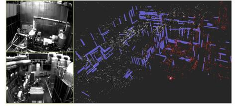
(c) **(Stereo)** Point-line map of *MH\_04\_difficult*. No planar structure due to the failure of CNN on this factory sequence. However, our map is as good as the map reconstructed from PL-VINS [10] which is a visual-inertial SLAM using points and lines.
