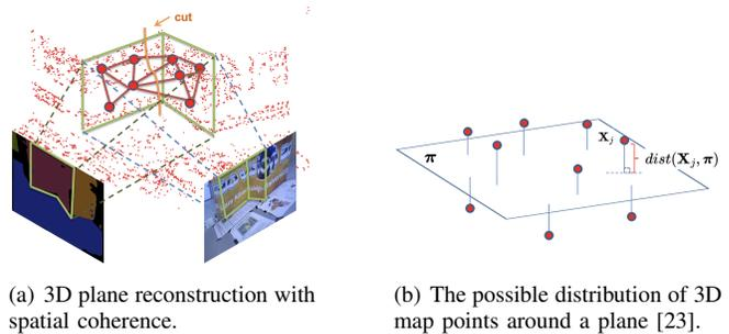
Fig. 3: **The interpretation of 3D plane:** (a) An example of 3D plane fitting optimized with spatial coherence. We initialize the plane by the given instance planar segmentation. Note that if two planes are wrongly segmented as one (e.g. due to texture similarity), they are separated later thanks to our graph-cut within a local neighborhood graph in 3D, as highlighted. (b) The possible distribution of the 3D points.
