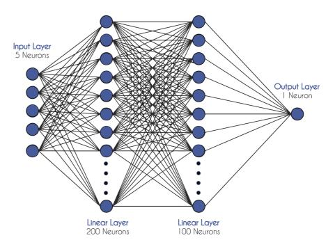
**Fig. 7** Neural network architecture for bacteria prediction
