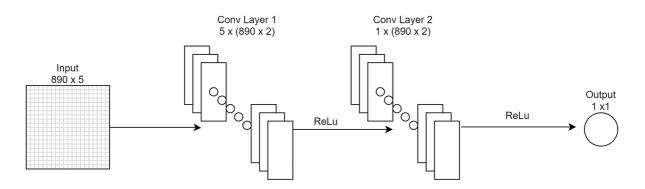
Fig. 8 CNN architecture for bacterial prediction
