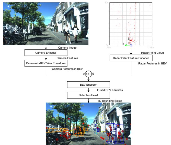
Fig. 1: Flowgraph of the presented radar-camera fusion in BEV, based on [5]. In the resulting camera image, we include projected radar detections and ground truth bounding boxes.
