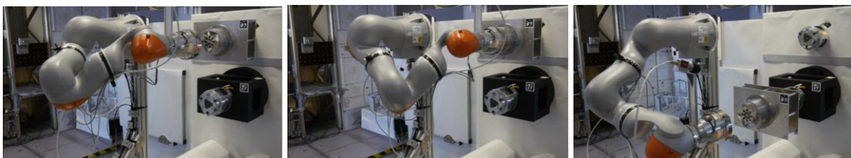
Figure 7 Tested mission sequence: Exchange of a payload equipped with two different standard interconnects. All available PERASPERA building blocks were integrated and demonstrated in this test-scenario: ESROCOS, ERGO, InFuse, i3DS and the two SIs SIROM and HOTDOCK. All elements were integrated in the AIRBUS RISMAT testbed.
