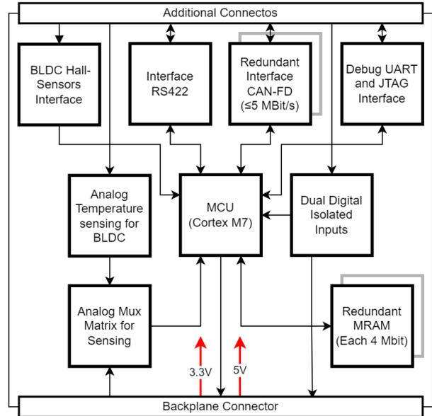
Fig. 4. The MCU board is the central unit for switching and control of the BLDC electronic and communication with a higher level system. It implements digital and analog interfaces for switching, control and sensing. Furthermore it is equipped with multiple interfaces for communication in operation and debugging. The MCU is based on a Cortex M7 with additional redundant external memory.
