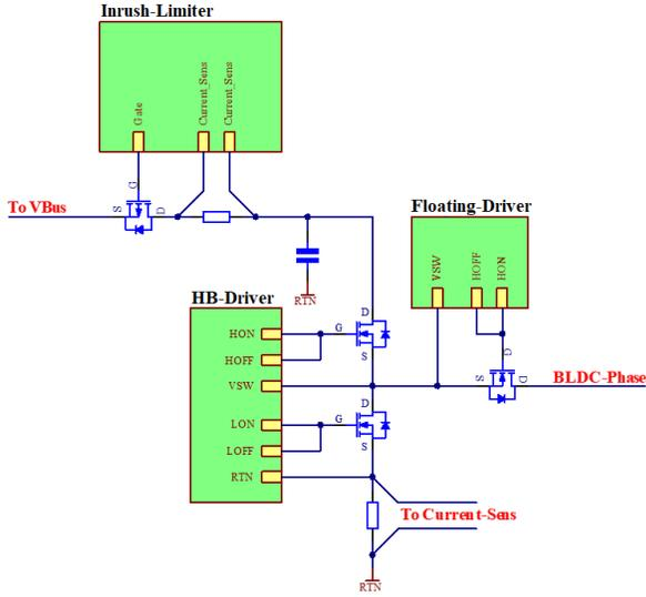
Fig. 3. BLDC fault isolation scheme. A PFET in the supply line and a additional GaN-FET per phase in serial make it possible to isolate a defective or redundant driver from a motor
