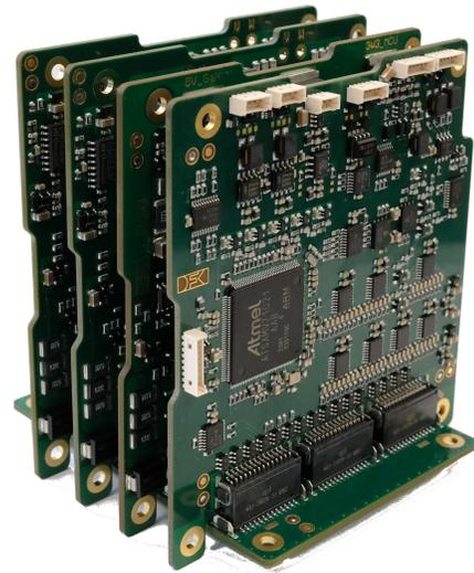
Fig. 1. Assembled modular BLDC power stage electronic consisting of the backplane and the connected MCU board, PSU board, and two cold redundant BLDC power stages.
