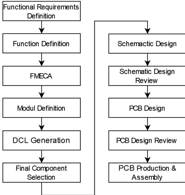
Fig. 2. The individual steps of the component selection and design process start from the definition of the functional requirements through the final selection of the components and finally to the design and manufacture of the electronics.
