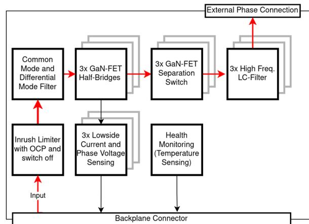
Fig. 6. The BLDC power stage board is supplied with 28 Vdc via the backplane. It has an inrush limiter with over current protection and switch off functionality. The power stage implements a common-mode and differential mode filter (see section IV). Each phase can be separated and is filtered with a high frequency LC-filter. There is a low-side current and phase voltage measurement for each phase. The external phase connection is on the upper side of the PCB and is not over the backplane.
