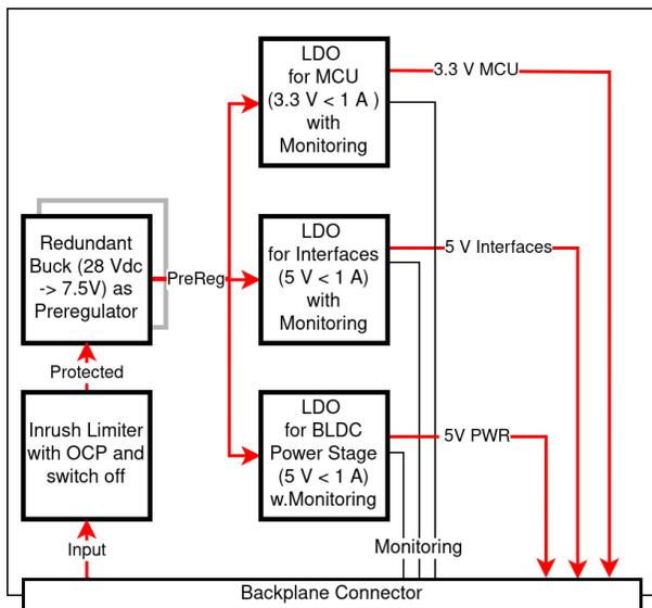
Fig. 5. The PSU board is directly connected to the 28 Vdc. It has an inrush current limiter that can also serve as a disconnecter. Two redundant switching power supplies (buck / step-down topology) in hot or cold redundancy (user-defined) serve as pre-regulators and generate approximately 7.5 V output voltage from the 28 Vdc. These 7.5 V are converted via LDO to 1x 3.3 V (for the MCU) and 2x 5 V (for the interfaces such as CAN bus, and RS422 and separately for the power output stage).
