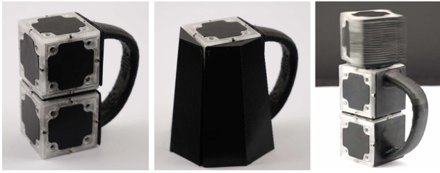
Figure 12: VoxelHap mug. BaseVoxel, VibrationVoxel and a mug handle using ShapePlates. Full shape resolution using ShapePlates. Added RotationVoxel and WeightPlate for moving mass simulation (left to right).
