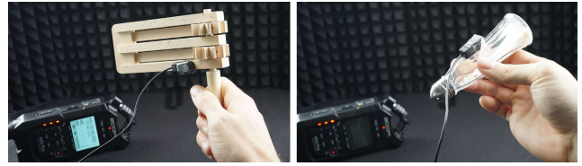
Figure 13: Recording vibrations from real-world object interactions using a condenser vibration pickup microphone.
