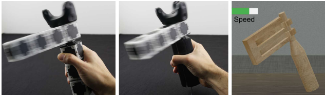
Figure 8: VoxelHap rattle. Low shape fidelity, high shape fidelity and corresponding virtual model (left to right).
