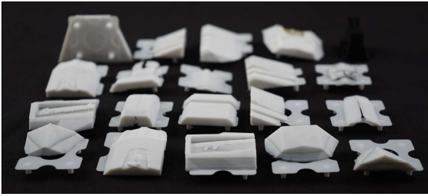
Figure 5: 3D-printed ShapePlates of the drill that can be attached to the low fidelity drill to increase shape resolution.
