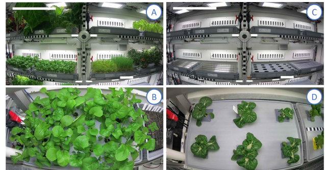
Figure 3: Exemplary neural network training images: (A) EDEN ISS side-view image showing arugula selvatica plants; (B) EDEN ISS top-view image showing arugula selvatica plants; (C) EDEN ISS greenhouse image without plants; (D) EDEN ISS top-view image showing Brassica rapa ssp. narinosa plants.
