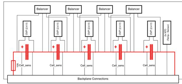
Fig. 6. The schematic diagram represents a CapBank module. In each instance, 5 supercapacitors, each of the 50F are connected to form a parallel network with its own overvoltage protection. Alternating across two of these arrangements are balancers. A 10 A fuse is provided to protect the system.
