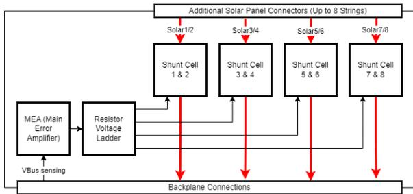
Fig. 5. The S3R does not contain a microcontroller. The control is done by a simple two-point controller that is controlled by an MEA which monitors the bus voltage and activates the individual shunt cells via voltage ladder if needed.
