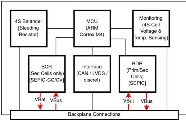
Fig. 7. A microcontroller provides central control and regulation of the charge and discharge controllers. If necessary, it can activate a passive “bleeding resistor” balancer. This module is universally designed, so that it is suitable for both primary and secondary cells.
