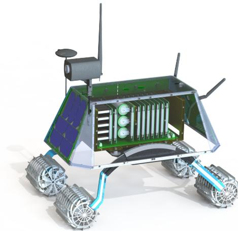
Fig. 1. Visualization of the MoVe rover with EPS inside. The rover serves as testbed for the EPS technologies developed within the project SEARCH
