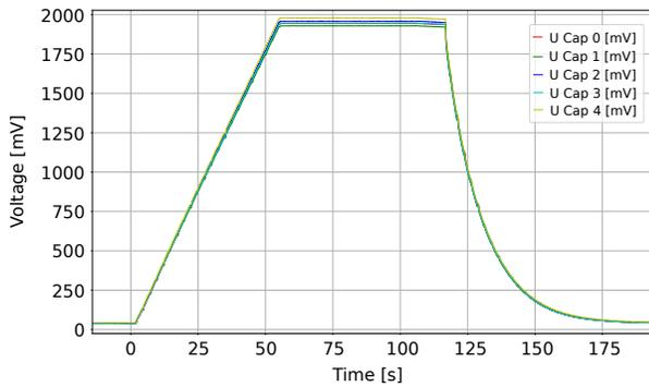
Fig. 8. 5 A charge test with modified CapBank. Full charge of the CapBank took at 5 A constant charge current around 55s.
