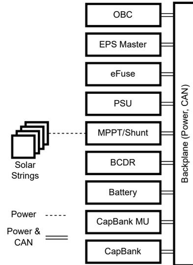
Fig. 3. The EPS and its components. It is comprised of multiple modules to implement the different functionalities for harvesting, storage, distribution, and control of power. The backplane provides power lanes and communication via CAN bus.
