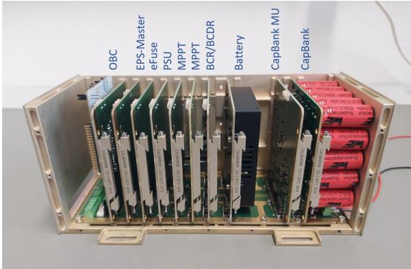
Fig. 2. Integration of the EPS. Cover and side panel removed for illustration. EPS including also supplementary modules as an OBC Board for controlling the rover, separate monitoring units for the CAP-Bank and the Battery module and an additional MPPT-Controller.
