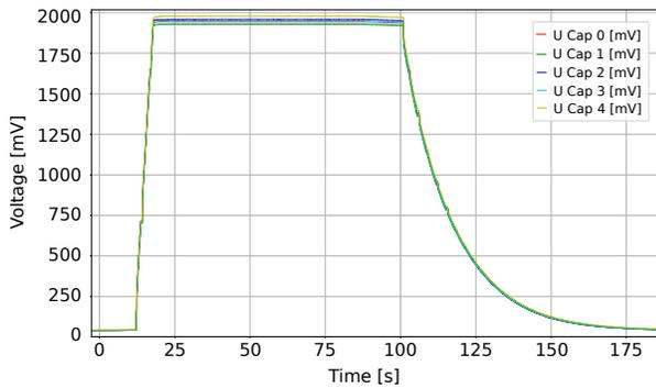
Fig. 9. 100 A charge test with modified CapBank. Full charge of the CapBank took at 100 A constant charge current around 8s. Also under these conditions the balancer keeps the voltage difference between the highest and lowest cell below 80 mV.
