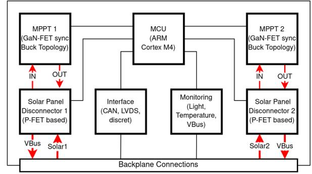
Fig. 4. The MPPT module consists of two identical channels controlled by a microcontroller. Since the solar panels have a higher voltage than the bus voltage of the rover, a synchronous buck topology based on GaN-FET was implemented.
