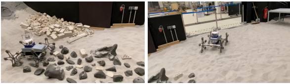
Figure 9: Field test setup for terrain classification.
