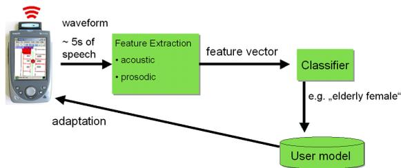
Figure 4: Integration into the M3I architecture
