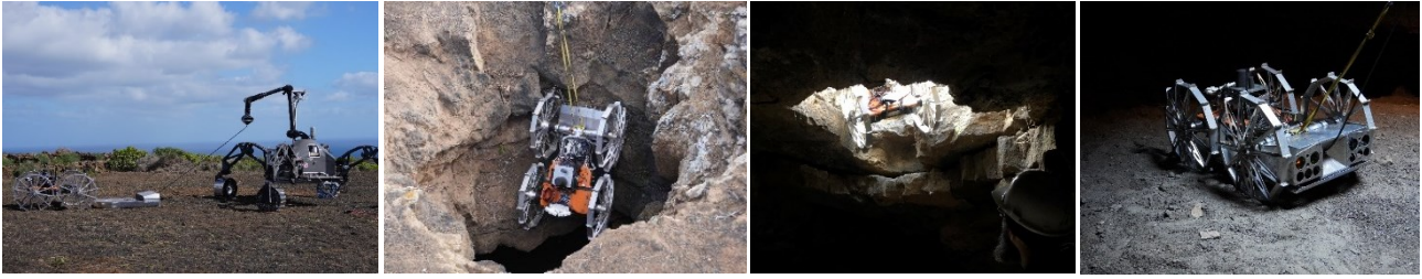
Figure 7 Several steps of Mission Phase 3 are depicted: Semi-autonomous docking between Coyote3 and the TMDS (left), descent of Coyote3 into the skylight (center-left), rappelling along the vertical walls (center-right) and touchdown at the bottom of the lava tube (right).
