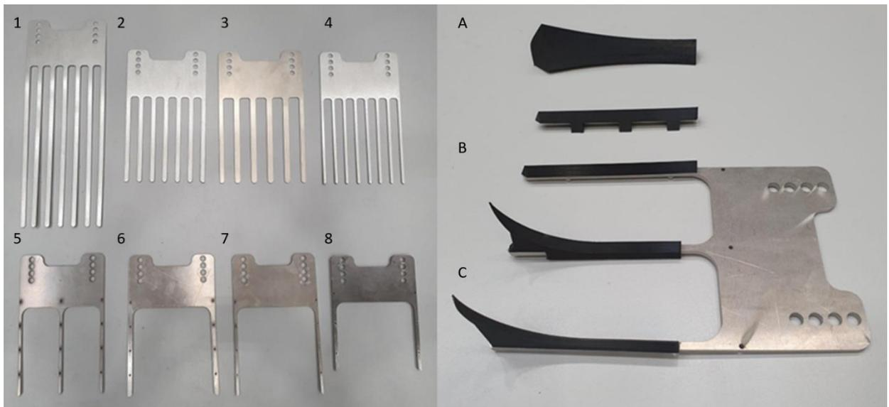
Figure 2: **Left:** Different holders for the attachments with various number of prongs, gap sizes, thickness and sinking depths (1-8); **Right:** Different attachments, from top to bottom: plough inspired design (A), two different wedges (B) and two bioinspired geometries (C).
