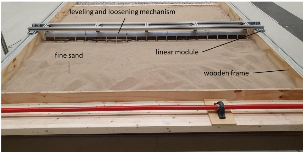
Figure 7: Ongoing integration of the mechanism into the test track
