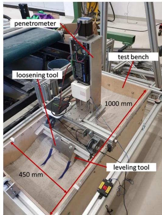
Figure 3: The test bench with penetrometer.
