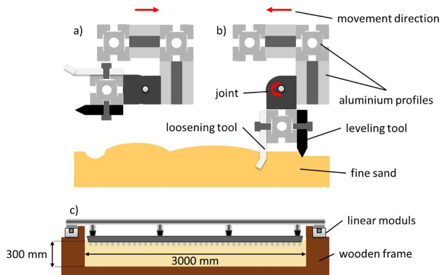
Figure 1: Concept of the mechanism; **a)** Movement forth with mechanism lifted; **b)** Movement back with tools in the sand for leveling and loosening; **c)** Mechanism attached on the test track.
