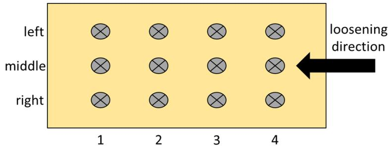
Figure 4: Description of measurement positions in the test bench for the loosening experiment
