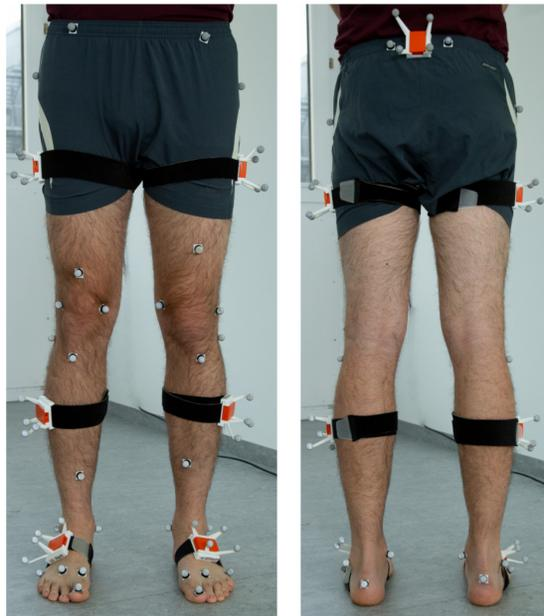
**Figure 8.** Experimental setup of the TUK-6-minute-walking dataset with IMUs and optical markers.
