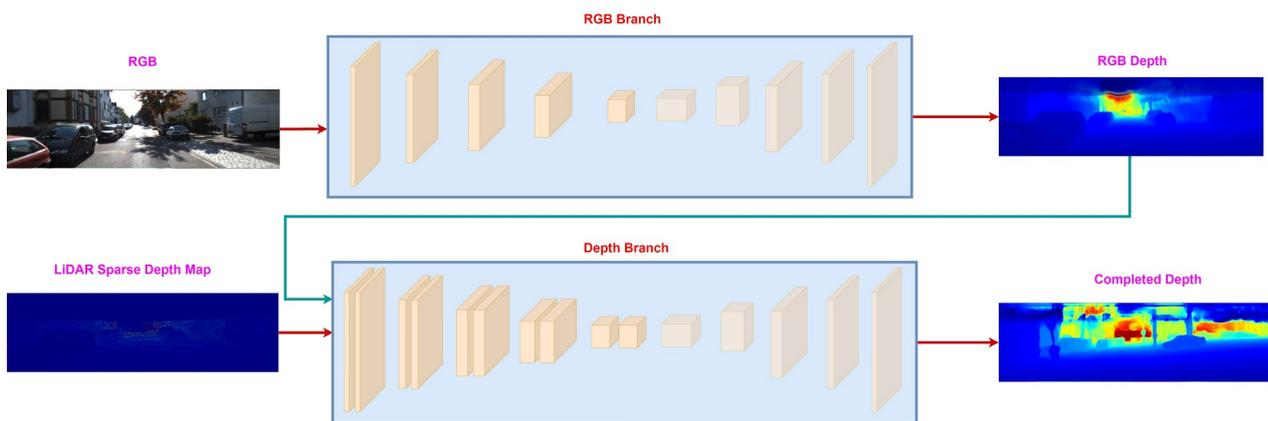
**Figure 4.** Sequential fusion between RGB image and LiDAR sparse depth map. The RGB branch produces color depth, which along with LiDAR sparse depth map, is sent to the depth branch to estimate the final dense depth map.
