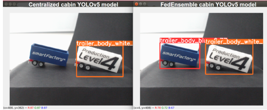
Fig. 11. Comparison of models trained using normal YOLOv5 (left) Federated Ensemble YOLOv5 (right) when the object (trailer attached to a chassis) orientation is not similar to the training images
