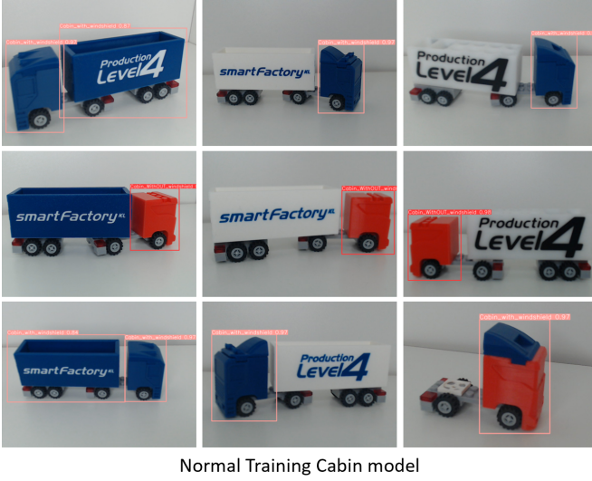
Fig. 6. Output of cabin model trained with Normal YOLOv5 algorithm on cabins assembled with different trailer types
