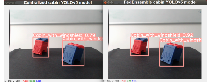
Fig. 5. Comparison of models trained using normal YOLOv5 (left) vs FedEnsemble YOLOv5 (right) when object has a different combination not present in the dataset (Cabin with different color type windshield without chassis)
