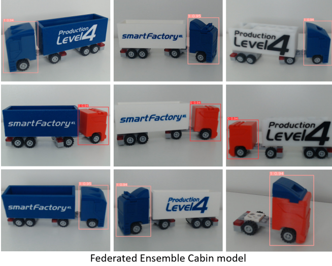
Fig. 7. Output of cabin model trained with Federated Ensemble YOLOv5 algorithm on cabins assembled with different trailer types
