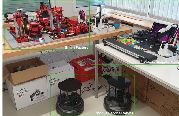
**Fig. 5.** Extended smart manufacturing setup with new CPS.
