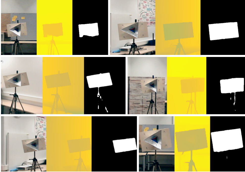
Fig. 14: Examples of the prompt bounding box calculated from the radar projection. The depth estimation shows a clear distinction between the foreground and the background and the instance segmentation results in a target mask for the camera-radar correspondences.
