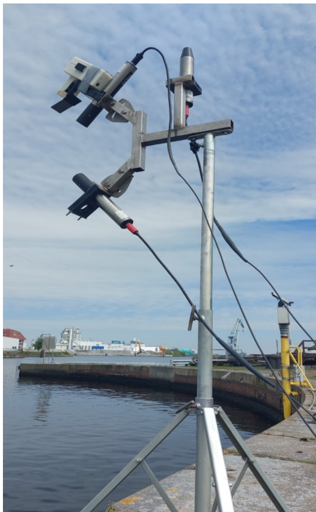
Figure 12. System set-up for a practical handling study assessing the field deployment of the EOW-RPI sensor system integrated with a hyperspectral radiometric measurement system.
