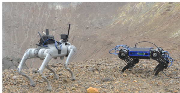
Figure 1. The control framework was successfully tested on both a Unitree Go2 robot and the custom build quadrupedal robot B12 during a field test on Vulcano Island in Italy.
