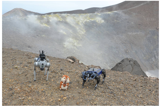
Figure 1. Two quadrupedal robots used during the field tests on Vulcano: Unitree Go2 (left) and Custom built B12 (right).
