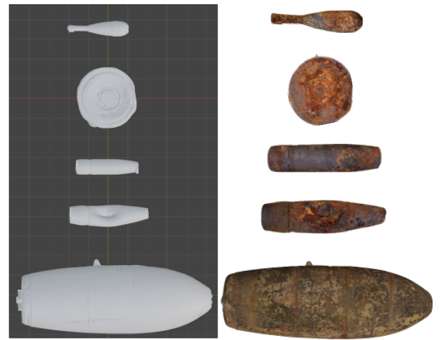
Fig. 2. Top-down view of UXO object meshes and corresponding real-life imagery. Left: meshes used in this work, from top to bottom: mortar shell, mine, artillery shell, deformed artillery shell, and 500 lb aircraft bomb; right: real-life images showing the rusted state of the corresponding UXO objects.
