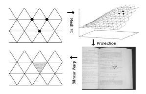
Figure 4: Image Dewarping. For a triangle within the planar mesh (top left), the 3D coordinates of its edges in 3D space (top right) are projected to the original image. The resulting triangle defines the texture patch (bottom right) which is warped bilinearly to its target position (bottom left).
