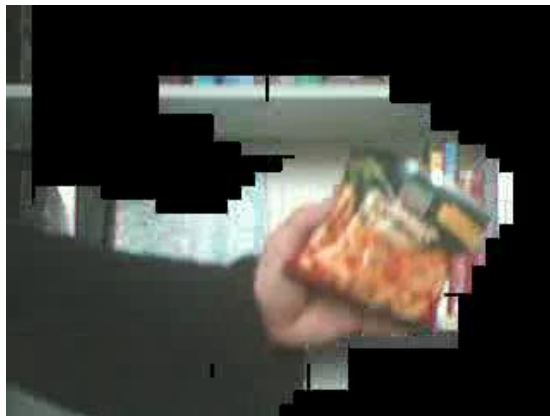
Figure 11: a typical motion segmentation result. The foreground does not only contain the object (as would be perfect for recognition) but also the operator's arm – which is correct, because it moves – and parts the background resulting from motion segmentation errors.
