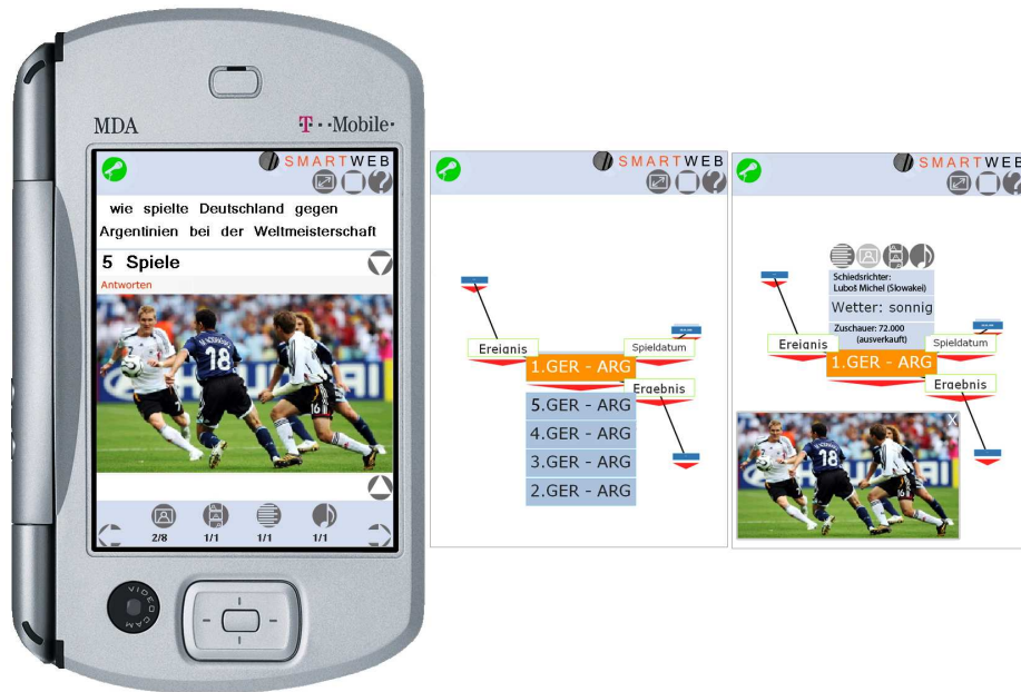
Fig. 1. SMARTWEB's main graphical user interface (left) and semantic navigation interactions (centre and right). By clicking on a certain vertex of the graph, the user can change the focus point for the fisheye distortion. With a click on the red arrow, the user can change an active instance . Clicking again on an active instance is an interaction form to ask for additional detailed multimodal information. When the structure of the dynamic graph changes, a new optimal layout is computed server-side. A further click on the Ergebnis (result) node results in displaying the information: 5:3 n. E., 1:1 n. V. (1:1, 0:0), Ereignis (incidence) reveals red card for player Cufre , for example.
