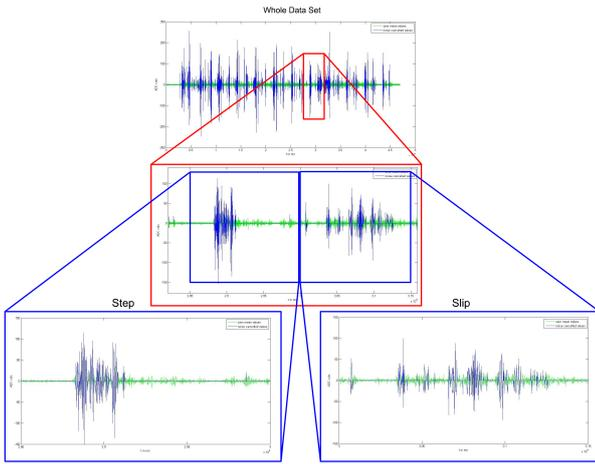
Fig. 11. Slip data of an experiment with the scout in the TestBed. Plotted are ADC ( $\pm 1.2g$  digitalized by a 10bit ADC) values against time. On top there is the whole data set from the one-minute experiment. In the middle, a frame with data from a step, and the following slippage, at the bottom of the picture a comparison of both data sets can be seen in a 1.5 second frame each.
