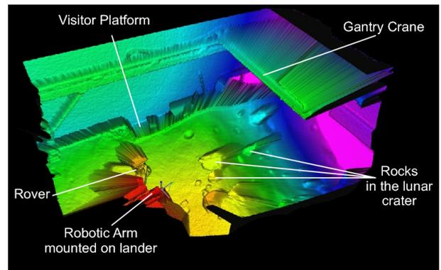
Fig. 3. 3D scan of the TestBed, taken from the sensor tower of the lander. A part of the lander with folded arm and the rover can be identified. The range of the laser scanner is sufficient to scan the whole TestBed, thus the gentry crane and the slope of the crater can be seen in the picture.
