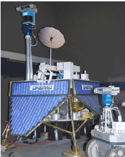
Fig. 2. Rover and landing unit in the test environment. On the lander mock up there is mounted a sensor tower with a 3D-laser scanner. A robotic arm is utilized for equipping the rover with different payloads.
