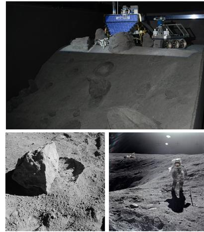
Fig. 1. The Crater Test Environment in comparison to moon pictures from NASA (Apollo 16), a flashlight was used to show the inner crater content, which otherwise would be too dark for the camera.
