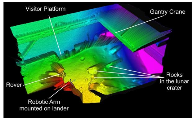
Fig. 3. 3D scan of the TestBed, taken from the sensor tower of the lander. A part of the lander with folded arm and the rover can be identified. The range of the laser scanner is sufficient to scan the whole TestBed, thus the gantry crane and the slope of the crater can be seen in the picture.
