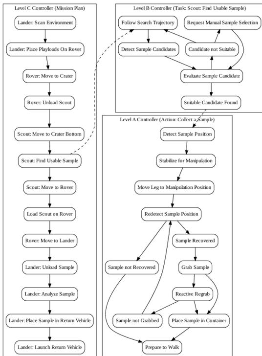
Fig. 6. Example of the Mission Control divided into Level C: Mission, Level B: Tasks and Level A: Actions. For Level B and A, one example is depicted in more detail.
