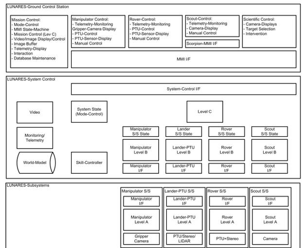
Fig. 7. Overview of the LUNARES control architecture: Bottom: Subsystem control with all level A controllers of rover, scout, lander, and manipulator. Middle: System control with level B and C, and other support functions like monitoring, telemetry, vision server, world model and skill controller. Top: LUNARES ground control distributed over several workstations.
