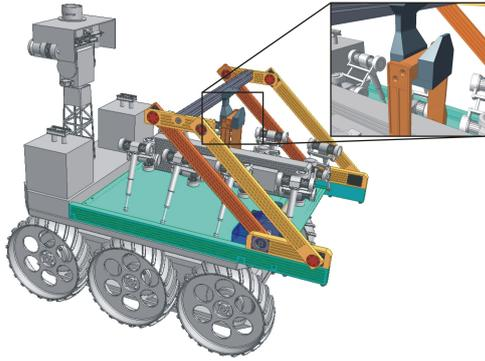
Fig. 4. CAD model of rover with docked scout. The docking adapter is realized as a parallel crank lever, allowing to keep the scout parallel to the cargo bay of the rover. The docking is passive by means of a hook and a bail.
