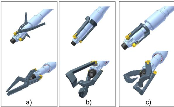
Fig. 12. Three different versions of Scorpion's claws. Experiments showed the clearance between shaft and tip of the first claw to be too great for damage free climbing in very rough terrain.
