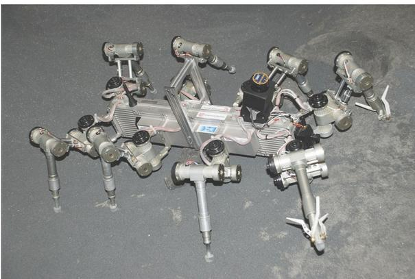
Fig. 5. The eight-legged scout "Scorpion". Each leg has 3 active DOFs and is equipped with an elastic spring component in the shank which is also used for ground contact detection. On the front legs there are mounted grippers used for sample acquisition.
