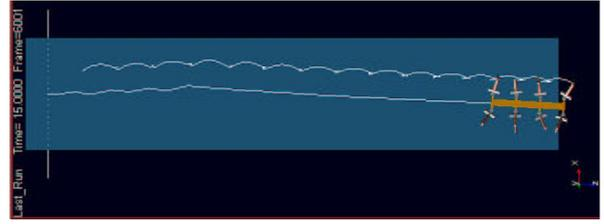
Fig. 10. Movements of feet relative to SCORPION's body, from [21]. The movement of feet in circular arcs around the body leads to increased bracing which in turn leads to increased slippage. By establishing an inverse kinematic layer, we are now able to easily move the feet parallel to the body.
