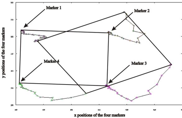
Fig. 9. Positions of the markers in the image plane tracked during the visual servoing process.
