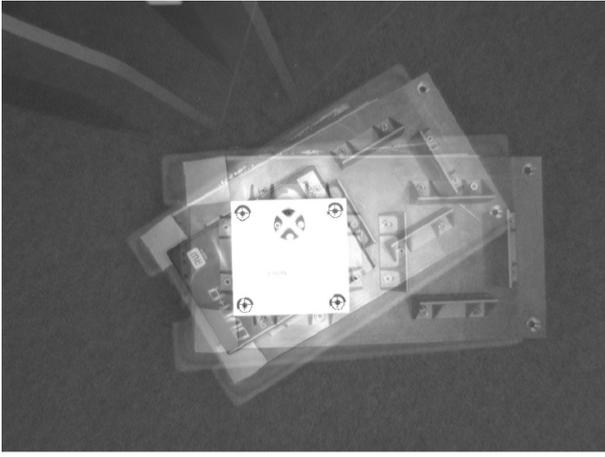
Fig. 8. Overlay of the reference image used for the teaching process of the Jacobian and the image of the camera view after successful control of the manipulator. The visual servoing was able to perfectly align the marker locations whereas the differences of the background clearly show the different situations.
