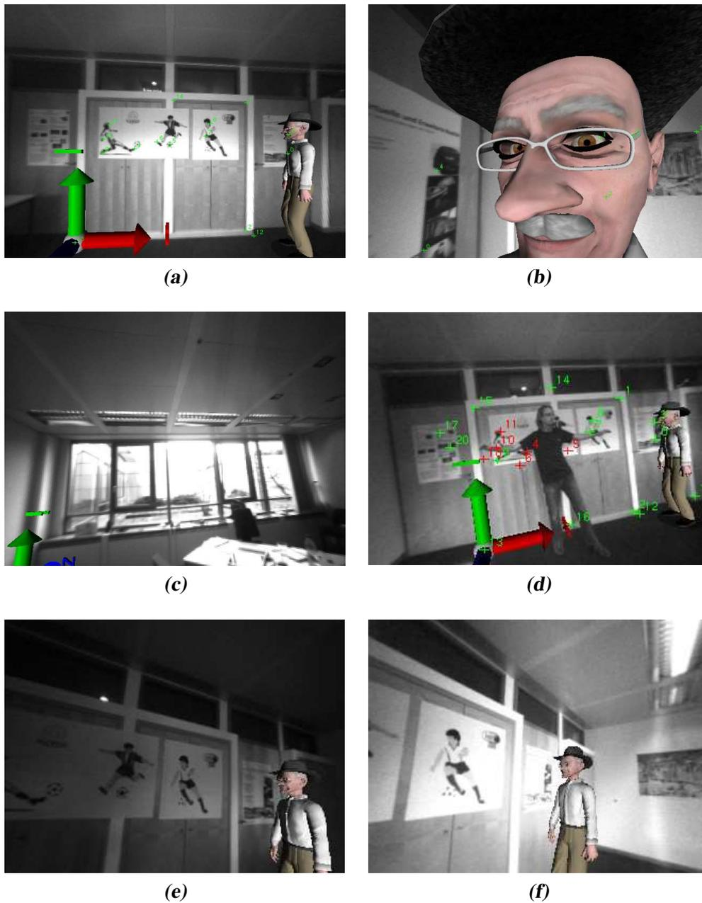
**Figure 3.14:** Room: some augmented frames demonstrating the range of possible movements (a-c) and the stable operation of the system under occlusion (d) and varying light conditions (d,f). Note that the wall observed in (c) is not part of the model. However, the augmentation in the lower left corner stays in its place. In (d) the green crosses indicate registered features and the red ones mark features where the registration failed due to the occlusion.
