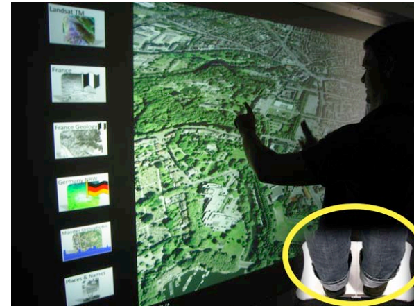
Figure 1: User is interacting with both hands and feet with a virtual globe using a large size multi-touch wall. User is standing on a Wii balance board (marked with yellow circle).
