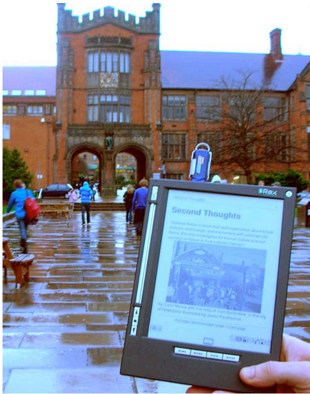
Figure 1: The iBookmark eBook reader. A GPS unit is attached to the reader for actual sensing various context variables based on the location of the users. Stories read by users on our modified eBook reader evolve and change every time a user reads at a different location. Here, the title adapts based on the current location. A photograph of the location is used on title page and, a result of the story, an “alien spaceship” is composited in the image.
