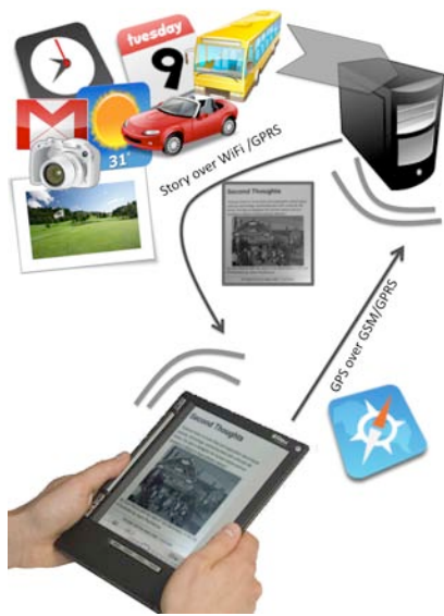
Figure 2.: The iBookmark system architecture. The eBook reader sends its current location to a server over GPRS to create stories that change in response to various context variables derived from the location.
