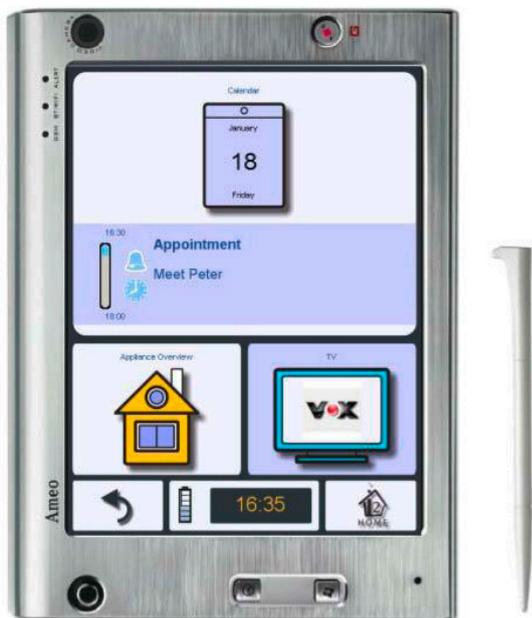
**Figure 4:** The i2home user interface for multimodal interaction on a smartphone
