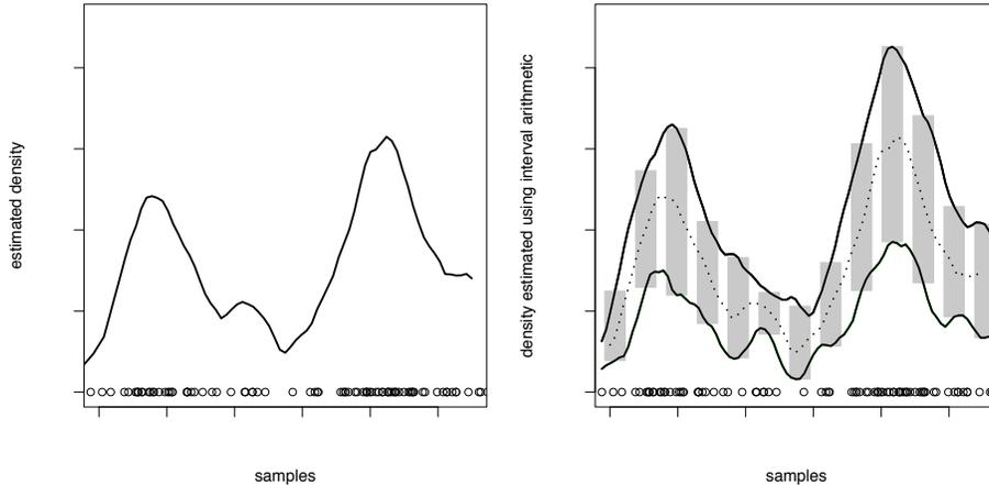
(a) A 1D kernel density with Epanechnikov kernel evaluated in conventional arithmetic. (b) The same kernel density as in Fig. 1(a) with Epanechnikov kernel evaluated using interval arithmetic
