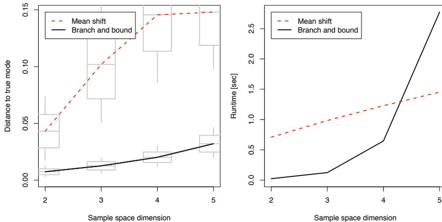
(a) Our method outperforms mean shift for mode finding in all tested dimensions. (b) For dimensions smaller than 5, mean shift is slower than the branch and bound algorithm.
