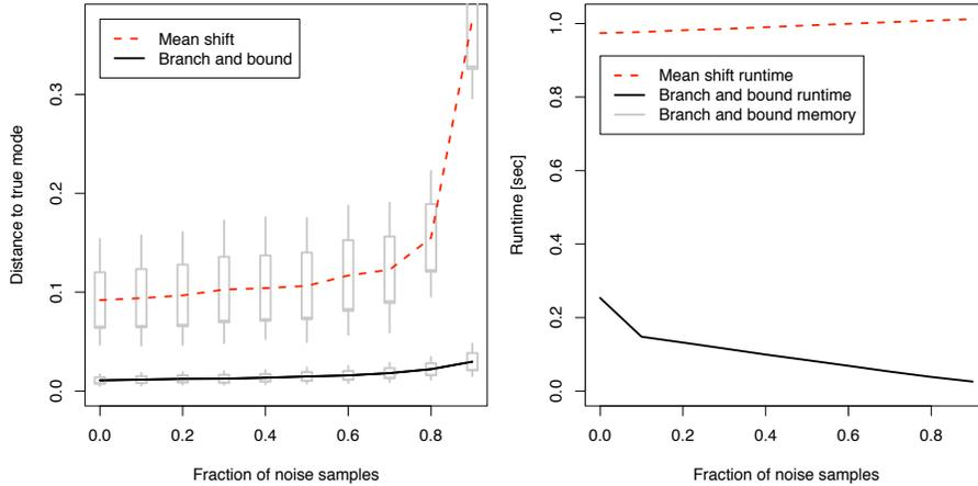
(a) Branch and bound mode finding is less sensitive to noise than mean shift. (b) Runtime of our method is significantly lower.
