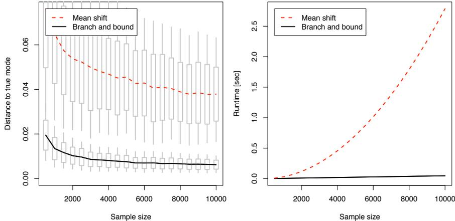
(a) Localization of our method is significantly better and converges faster than the one of mean shift. (b) In contrast to mean shift, branch and bound mode finding scales linearly with samples size.
