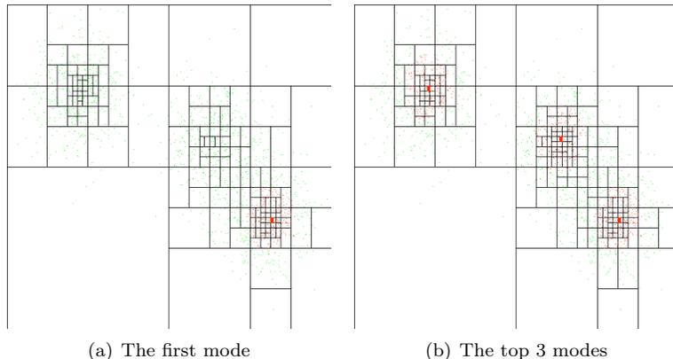
Figure 2: Examples of applying the adaptive subdivision to some 2D data. Data samples are shown as green points. Red points indicate samples that had a non-zero contribution to the kernel density at the final intervals (“active samples”).
