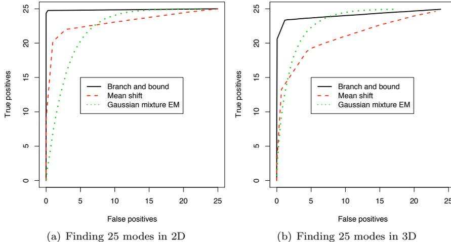
Figure 6: Experiments with samples from a 25-Gaussian mixture ( $\sigma = 0.25$ ) and 50% noise fraction. The total number of points was fixed to 5000. To measure these ROCs, the distance at which a true mode was counted as matching an estimated one was varied.
