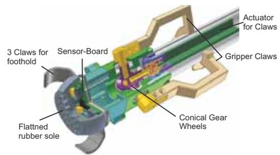
**Figure 12:** Second prototype of the intelligent SpaceClimber foot
