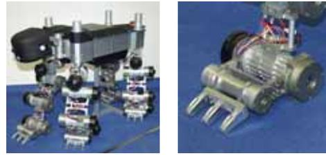
**Figure 3:** Aramies robot and foot with actuated claw
