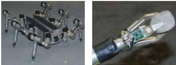
**Figure 2:** Scarabaeus with feet enabling sampling
