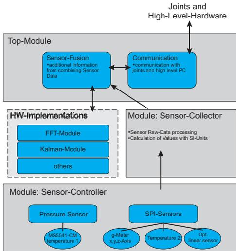
**Figure 9:** Layout of FPGA hardware design.
