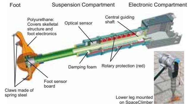
**Figure 8:** Description of SpaceClimber's lower leg. Bottom right displays the leg mounted on the robot, visible cables are due to experimental data logging with external PC.
