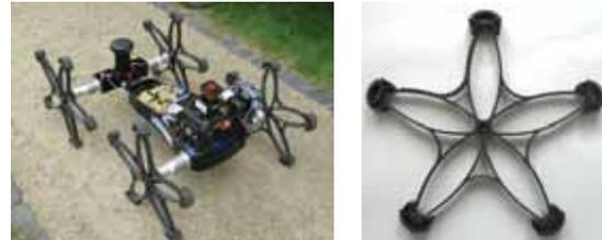
**Figure 6:** Asguard and compliant legged wheel
