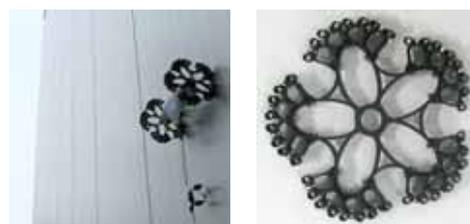
**Figure 7:** Magnet-Crawler and magnetic legged wheel
