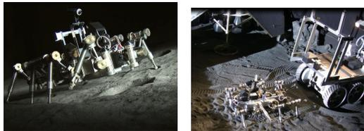
(e) Scout climbs back up to the rover (f) Scout docks to the rover, the rover commands the scout
