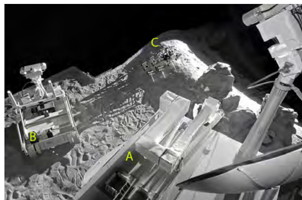
Figure 1. LUNARES systems: Landing unit (A), wheeled rover (B) and legged scout (C) in the artificial crater environment
