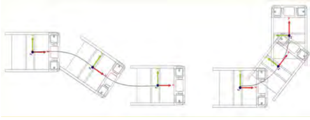
Figure 6. Cubic splines and circle segments are used to generate more complex trajectories for the rover
