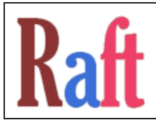
Figure 3: Example of how connected component extraction can fail. Here this image was recognized as containing three components 'R' 'a' and 'H'. The image is of the word 'Raft', but due to the font that it is typeset in and noise, the space between the 'f' and 't' is invisible. To a connected component extraction system, each horizontal white space delimited sequence of black pixels is considered a connected component.
