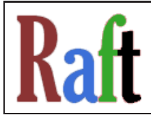
Figure 4: Example of how using a statistical language model can yield better results. Here this image was recognized as 'Raft' because 'RaH' could not be found commonly in a corpus of English text.
