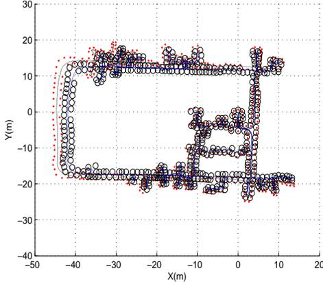
(b) The DLR data set: 3297 robot poses and 539 feature positions. Circle – feature estimate using identity covariance, dot – feature estimate using original covariance
