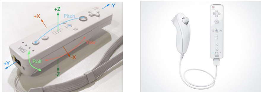
Fig. 2 Right: The WiiMote controller and Nunchuk. Left: Accelerometer axes.
