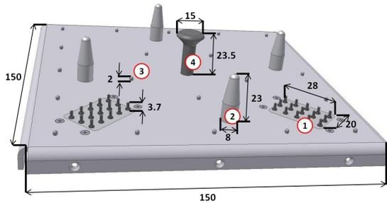
Fig. 6. Passive part of electromechanical interface on module top with dimensions in mm 1) Block of contact probes 2) Dome-shaped centering pins 3) Distance pins 4) Bolt for latch mechanism
