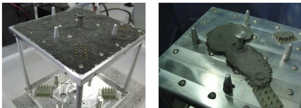
(a) Plain layer of rough dust (b) Rest of compressed fine dust after experimental trial
