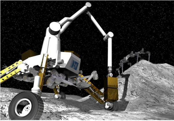
Fig. 1. Artist drawing of the RIMRES system. One legged scout is climbing a steep slope while a second is mounted beneath the rover. The wheeled rover is deploying a stack of two payload items on the surface.
