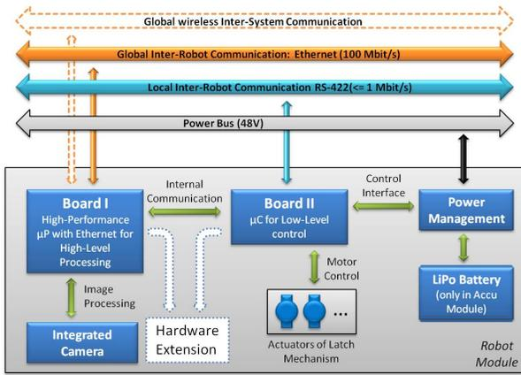
Fig. 3. Basic components in each module. The three bus systems energy, local communication via RS-422, and global communication via ethernet are provided by the electrical part of the EMI.
