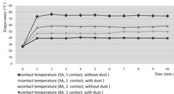
Fig. 9. Temperature of the contact probes
