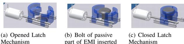
Fig. 4. Latch mechanism
