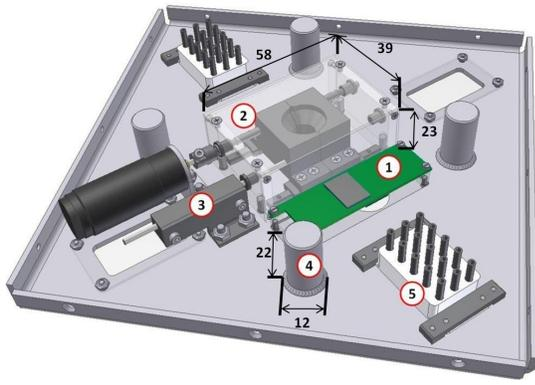
Fig. 5. Active part of electromechanical interface integrated in module bottom with dimensions in mm 1) Camera 2) Mechanical latch mechanism with spindle drive and dust protection housing 3) Linear potentiometer 4) Cylinder with conical mouth 5) Block of contact plates
