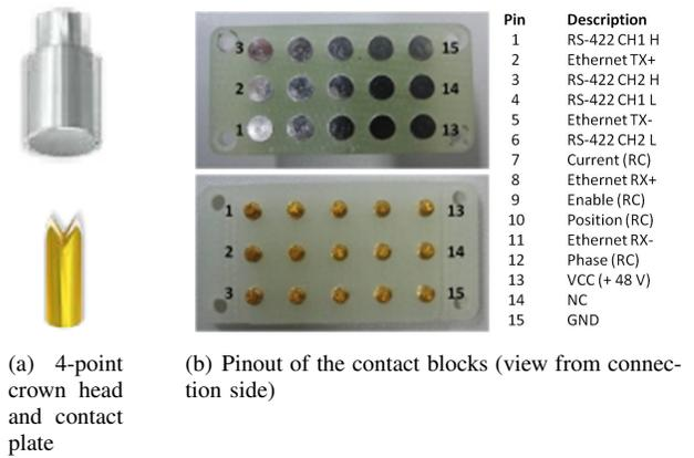
Fig. 7. Contacts and Pinout
