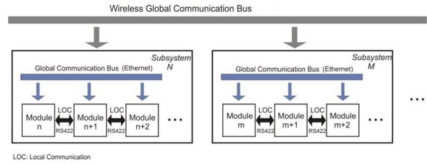
Fig. 2. Three communication levels in the RIMRES system: Modules can communicate with their direct neighbors via local communication (RS-422) (used for docking procedure and topology recovery), Ethernet is used for wired communication in a physically connected system. Wireless communication is employed between remote subsystems.
