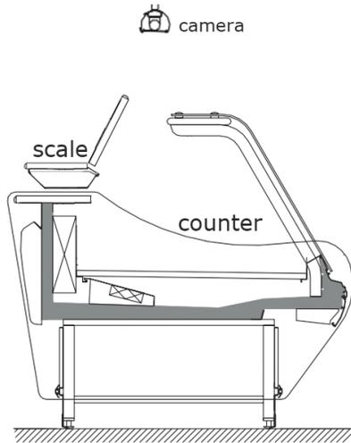
**Figure 3:** The figure shows the illustrated application setup with the counter, the scale with display for employee and customer and the Kinect mounted above the counter.
