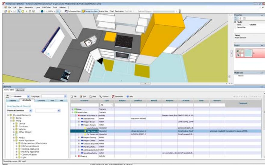
Figure 2. The design toolkit integrates a 3D model (upper frame) with a tabular activity model (lower frame), that uses ontological concepts (lower left).
