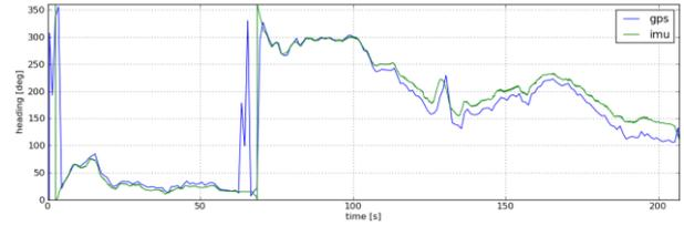
Figure 11. Heading estimate on the Asguard system.
