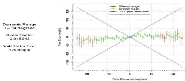
Figure 7. SEA Gyro Rate Error Plot
