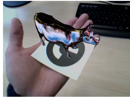
Fig. 1. Circular marker for Augmented Reality
