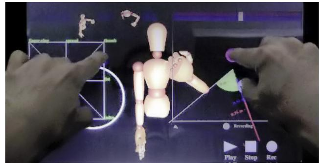
Figure 1: Our bimanual multitouch interface allows simultaneous control of the various degrees of freedom of a human arm.
