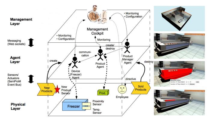
Figure 1. The architecture and communication channels for the implemented components (left) and screenshots of the visualization component (right).
