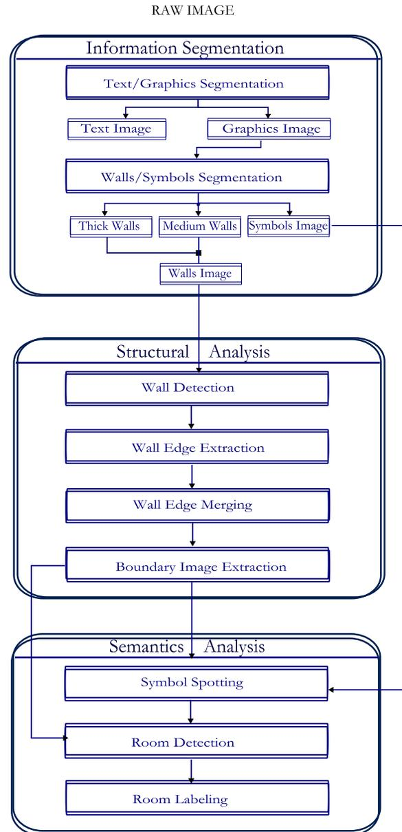
Figure 1: Automatic Floor Plan Analysis Workflow
