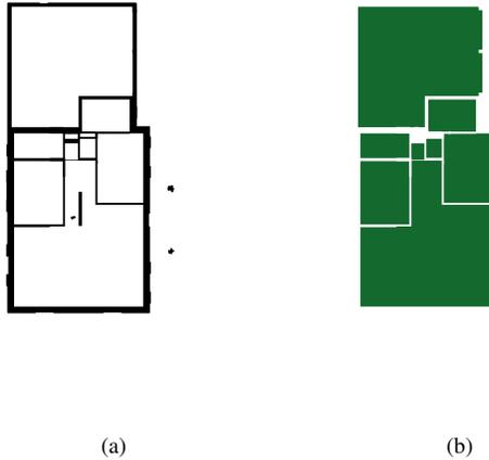
Figure 6: Room detection: floor plan image after closing the gaps at doors and windows (a) and the final room detection result (b)
