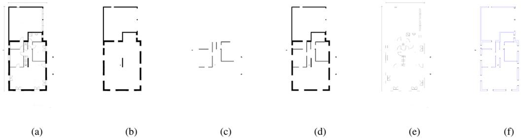
Figure 3: Walls/symbols segmentation of the floor plan illustrated in Fig. 2a: graphics image (a), extracted thick walls (b), medium walls (c), and combined walls (d); extracted symbols (e) and walls after contour and wall edge detection (f)
