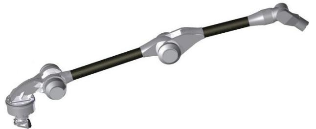
Fig. 8. Manipulator arm design based on optimization results. The left end is the first joint that is incorporated into the rover's central tower. The right end is the end effector without EMI.
