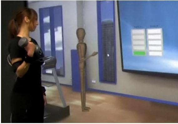
Fig. 4: The virtual trainer in use: The user exercises equipped with two IMUs on the arm in front of a big screen. The movements are transferred to an avatar in a virtual gym environment. The system counts the biceps curls and fills up green bars to indicate the number of repetitions.
