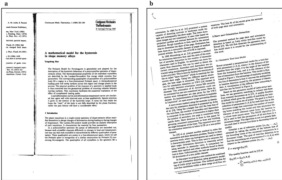
Fig. 1 Examples of scanned document images. a Straight, horizontal text-lines. b Skewed text-lines (8° skew angle)
