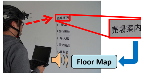
Figure 1. Translation camera system with a head-mounted eye-tracker.
